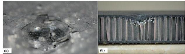
Fig. 8: Photo of indentation damage in sandwich panel after quasi-static indentation test showing (a) fiber breakage and cracking in face sheet and (b) core crushing and local buckling in cross sectional view
