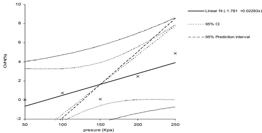
Figure 3. Hydraulic design's coefficient of variation of pressure-compensating emitters with respect to different operating pressure of water source.
