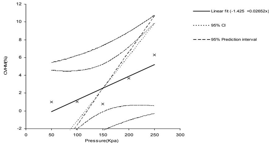
Figure 5. Total coefficient of variation of pressure-compensating emitters with respect to different operating pressure of water source.
