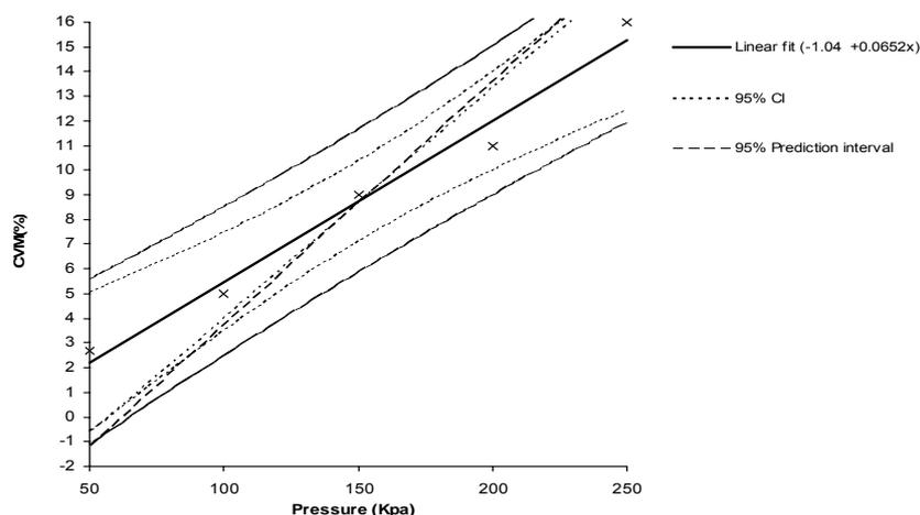
Figure 2. Manufacturer's coefficient of variation of non pressure-compensating emitters with respect to different operating pressure of water source
