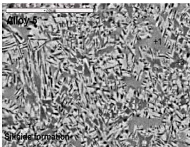
Figure 3. Precipitation in 3 mm thick bulk ingot of the alloy. Phases are marked.
