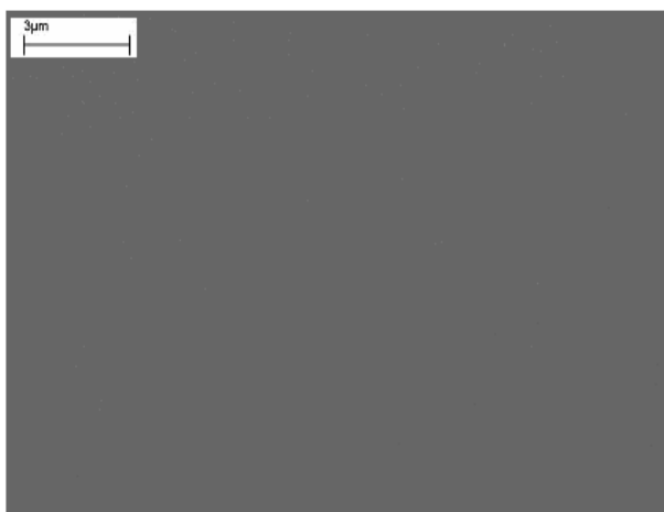
Figure 2. Featureless surface of 50 \mu\text{m} thick as-cast melt spun ribbon.
