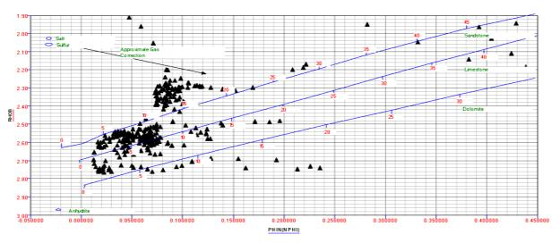
Fig. 6: NPHI-RHOB cross-plot showing lithology of the Hangu Formation modified after [13].
