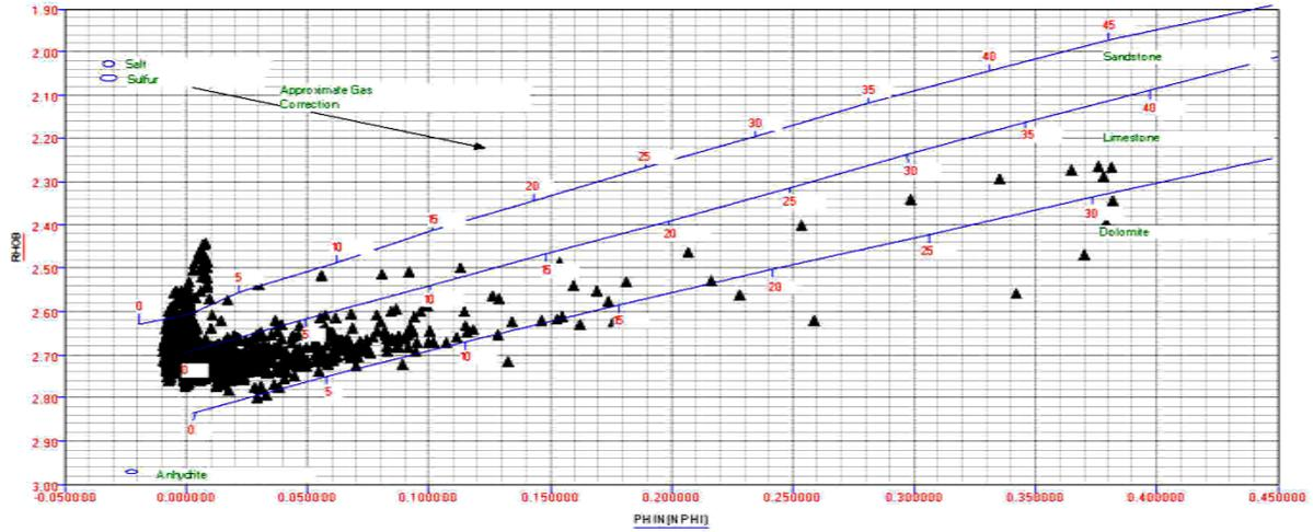
Fig. 5: NPHI-RHOB cross-plot showing lithology of the Lockhart Limestone modified after [13].
