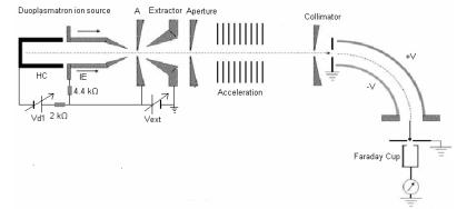
Figure 1. Schematic of experimental setup to analyze the energy of ion beam
