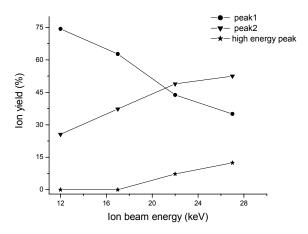
Figure 4. Trend of ion yield w.r.t ion beam energy.
