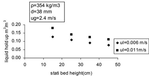
Figure 5b. Effect of static bed height on liquid holdup for type 2.
