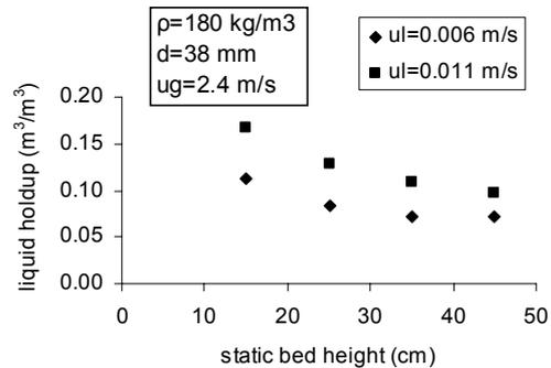
Figure 5a. Effect of static bed height on liquid holdup for type 1 fluidization
