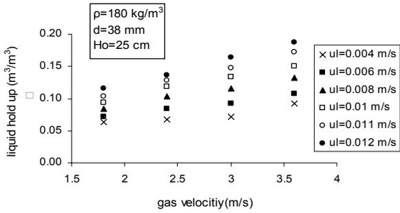
Figure 2. Effect of liquid and gas velocities on liquid hold up for type 1.
