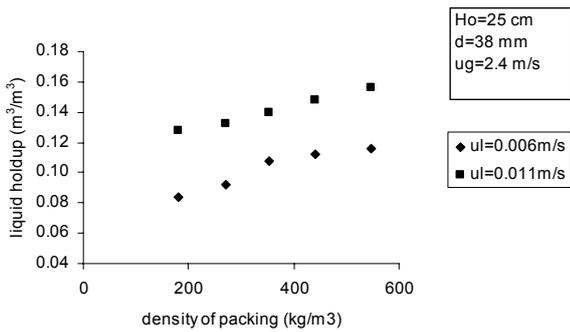
Figure 3. Effect of liquid and gas velocities on liquid hold up for type 1
