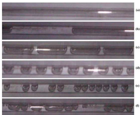
Figure 5. Observed flow patterns. (a) Annular flow; (b) Annular to Taylor transition; (c) Taylor flow; (d) Taylor to Bubbly transition; (e) Bubbly flow; (f) bubbly to churn transition
