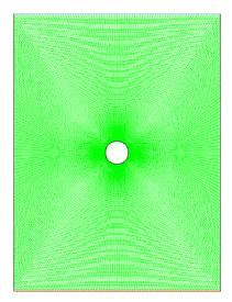
Figure 5. Schematic diagram of geometry for bubble of 1.5 mm diameter with structured mesh.
