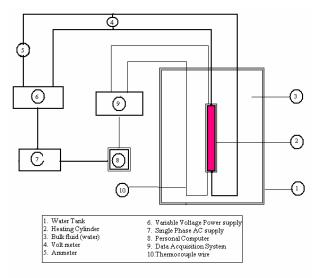
Figure 1. Schematic diagram of experimental setup.
