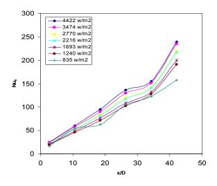
Figure 4. Local Nusselt number along dimensionless length x/D at different uniform heat fluxes.
