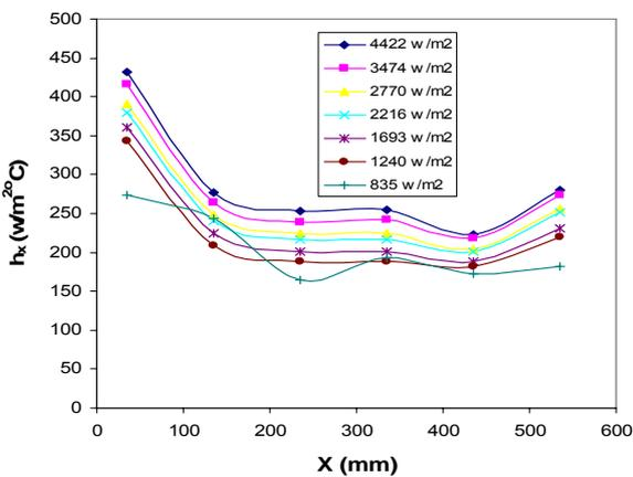
Figure 3. Local Heat Transfer Coefficient along axial distance at different uniform heat fluxes.
