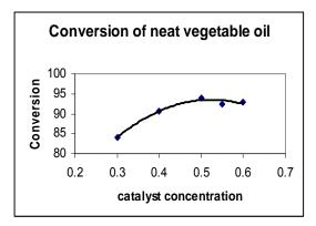
Figure 4. Effect of catalyst concentration on conversion of neat corn oil.
