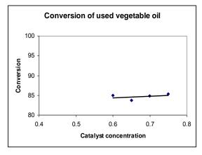
Figure 5. Effect of catalyst on conversion of used corn oil.
