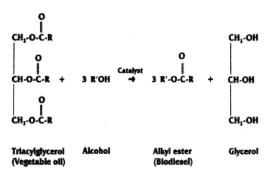
Figure 1. Transesterification Reaction.
