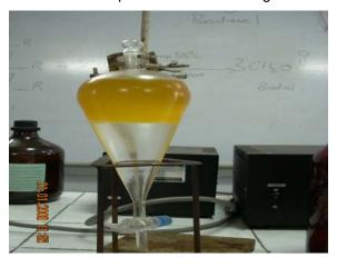
Figure 3. Washing of Biodiesel.
