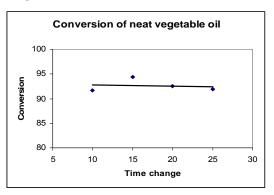
Figure 10. Effect of time on conversion of neat corn oil.
