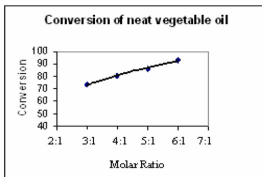
Figure 6. Effect of molar ratio on conversion of neat corn oil.
