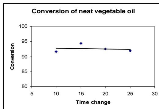
Figure 10. Effect of time on conversion of neat corn oil.
