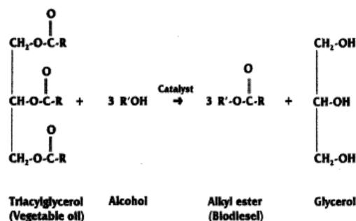
Figure 1. Transesterification Reaction.
