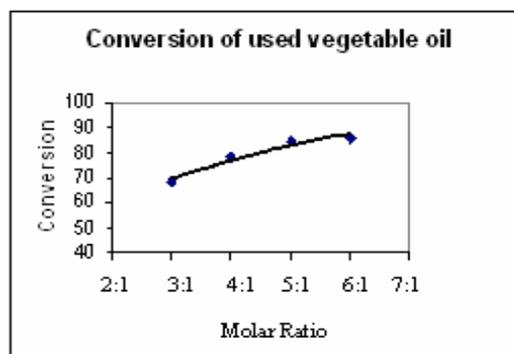
Figure 7. Effect of molar ratio on conversion of used corn oil.
