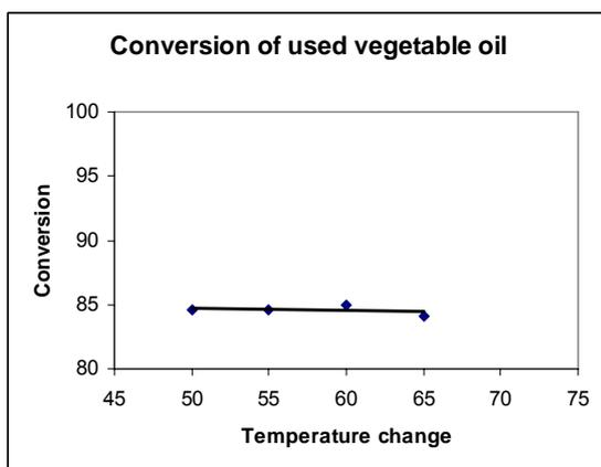
Figure 9. Effect of temperature change on conversion of used corn oil.
