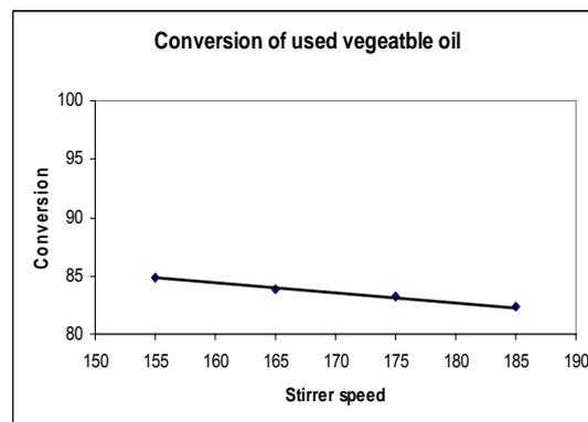
Figure 13. Effect of stirrer speed on conversion of used corn oil.
