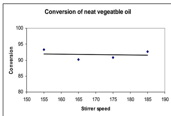
Figure 12. Effect of stirrer speed on conversion of neat corn oil.
