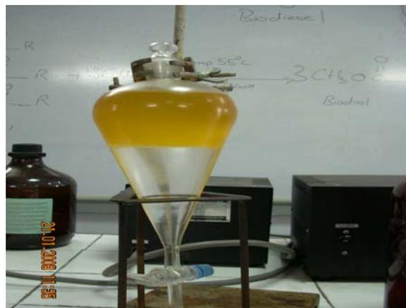
Figure 3. Washing of Biodiesel.
