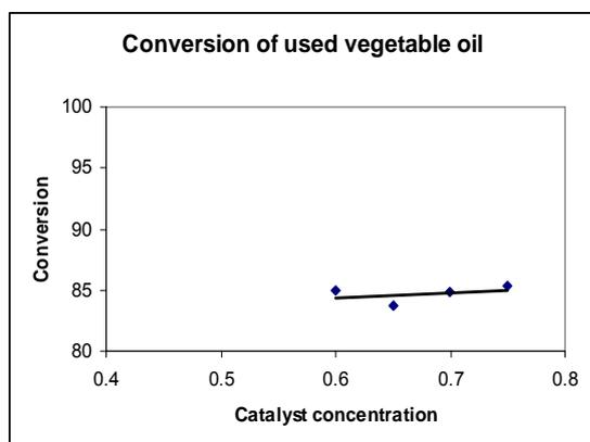
Figure 5. Effect of catalyst on conversion of used corn oil.
