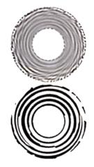
Figure 17. Simulation of a two-phase extrusion showing alternating concentric regions of each phase. Shown is the morphology after 1 s (top) and 20 s (bottom).
