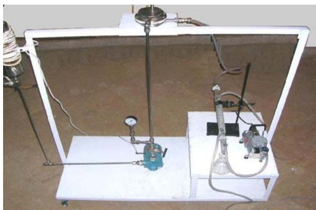
Pervaporation Rig Comprising Membrane Cell Fabricated and Assembled as part of MS Research Projects.
