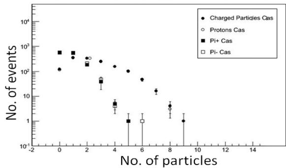
Fig. 4: The number of events as a function of charged particles produced in deuteron-carbon interactions from cascade code
