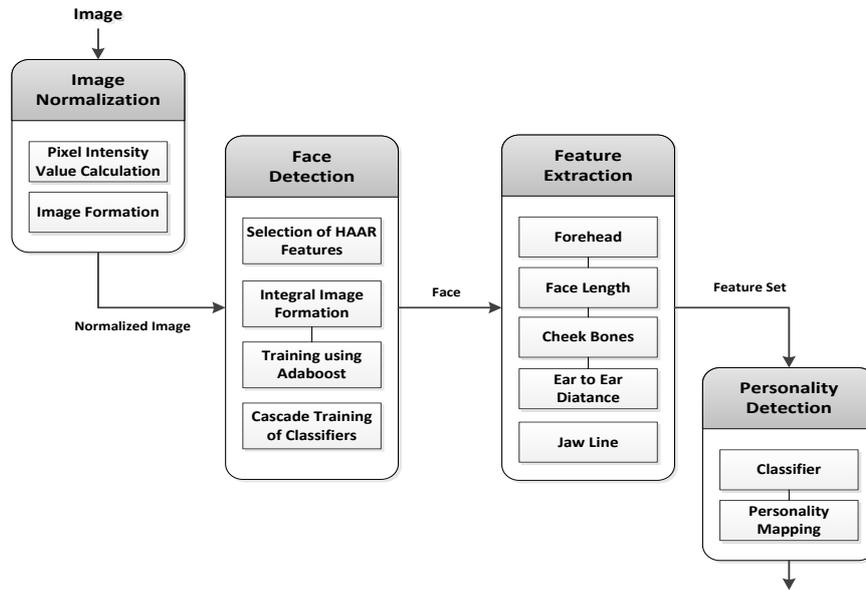
Fig. 4: Detailed description of the proposed algorithm
