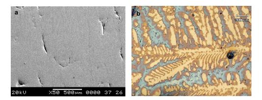
Figure 2. SEM and optical micrographs of as cast samples of Samarium-Cobalt (SmCo<sub>5</sub>). After polishing and etching shows (a) single phase microstructure (b) typical dendratric structure.
