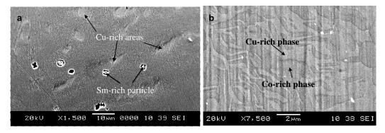
Figure 3. SEM micrographs of the sample  $SmCo_{1-x}Cu_x$  with x = 1.5 after polishing and etching. Samples reveal two-phase structures (a) as-cast (b) annealed at 800°C for 3hrs.
