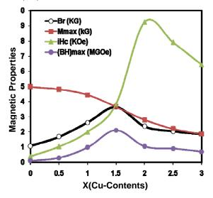
Figure 4. Magnetic properties of SmCo<sub>1-x</sub>Cu<sub>x</sub> as a function of copper contents.
