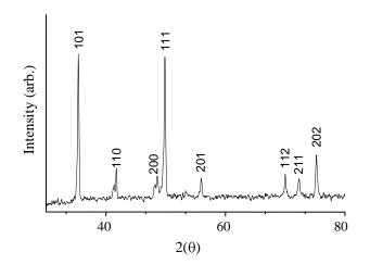
Figure 1. XRD pattern of as-cast SmCo<sub>5</sub> alloy.
