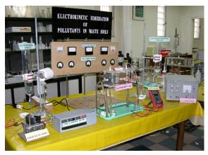
Figure 1. Laboratory setup for electrokinetic remediation of Cr in waste soils.
