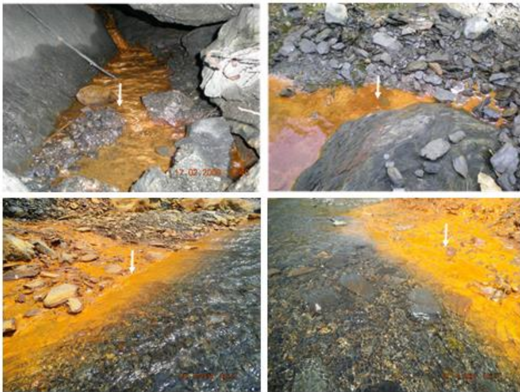
Fig. 2: Acid mine drainage representing bacterial oxidation of pyrite and sulfide minerals in the black shale formation of Chamiari (Ghazi Tarbela) and Kala Katha, Khyber Pakhtunkhwa (Pakistan). The arrows point at the formation of red-brownish Fe(III)-precipitation in the mine drainage.
