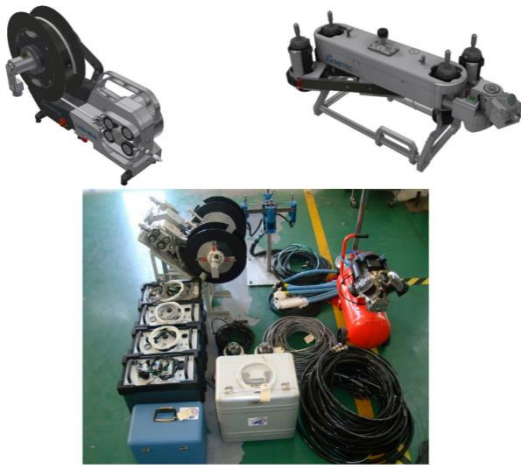
Fig. 9: Typical ET SG Tubes Inspection System
