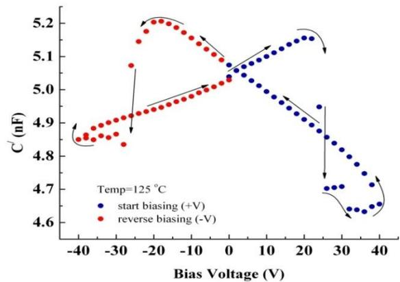
Fig. 3: Capacitance versus bias-voltage bipolar plot for [111]-oriented PMN-PT crystal measured at  $125^\circ\text{C}$  well inside the ferroelectric tetragonal phase
