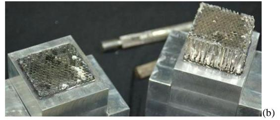
Fig. 5: a) Flatwise tensile strength comparison between neat and hybrid sandwich panels, b) photograph of failed sandwich sample showing adhesive failure
