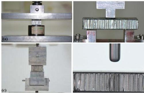
Fig. 2: Photos of test setups (a) Flatwise compression test (b) Flexural test (c) Flatwise tensile test (d) Quasi-static indentation test
